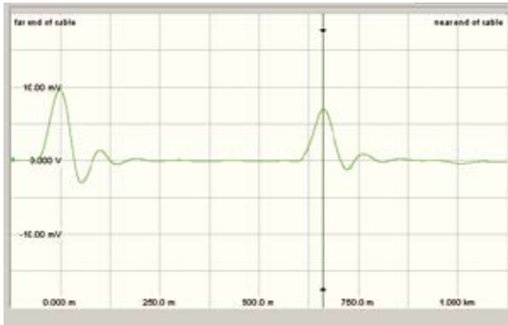
Runtime based fault location
